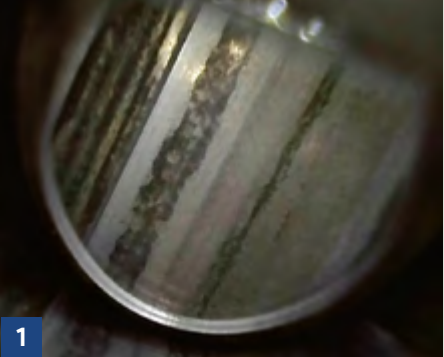
This image was taken after a solvent-soaked patch had already been pushed through the barrel. Even after one cleaning pass there's still fouling, solvent residue and patch fibres visible under magnification. It's a good reminder that one wet patch and a quick scrub usually isn't doing nearly as much as people think it is.
