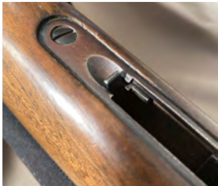
The recessed magazine release of the Brno Model 2, which is how the Zephyr's magazine release should be.
