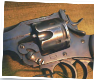
The cylinder on a Webley Mk VI service revolver (Image: Webley and Scott).
