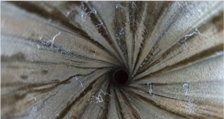
This image was taken after a solvent-soaked patch had already been pushed through the barrel. Even after one cleaning pass there's still fouling, solvent residue and patch fibres visible under magnification. It's a good reminder that one wet patch and a quick scrub usually isn't doing nearly as much as people think it is.
