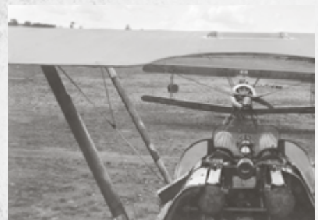
Cockpit view from inside a WWI Sopwith Camel fighter, showing the two Vickers .303 machine guns, which fired through the propeller.
