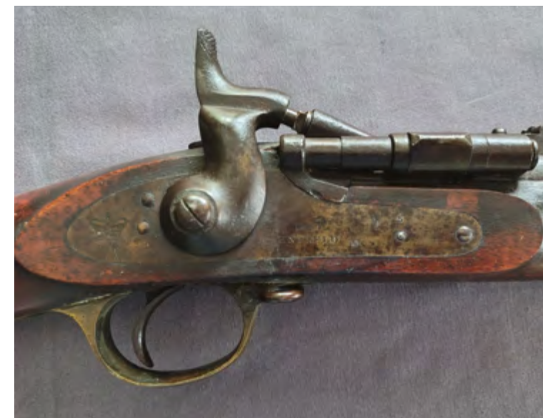
An Enfield Pattern 1853 muzzle loader that was converted to a breech loader in the 1860s. This rifle saw service in Canada.
