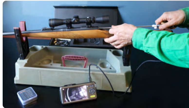
The NTG200H + NTS500B bundle in use; rifle bore examination is easy using the rigid scope probe and the high-resolution monitor.
