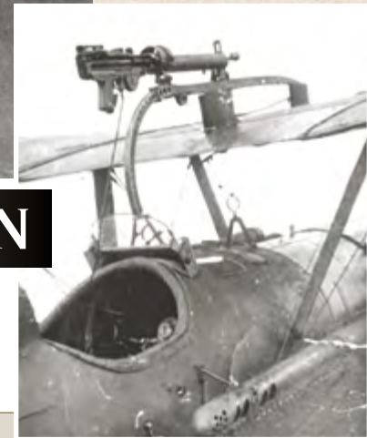
Foster mounting for a Lewis Mk II on an SE5a fighter.
