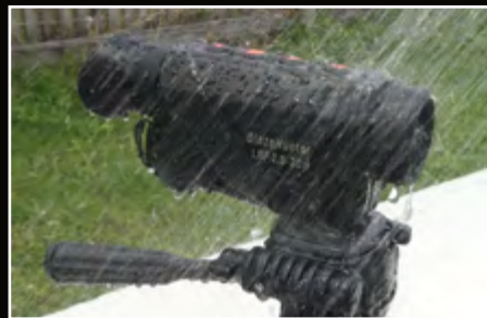
Spraying the unit with a hose while turned on didn't cause any problems thanks to its IP67 rating.
