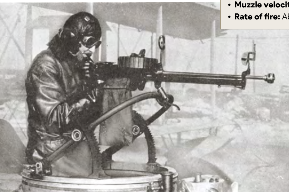
Flexible Lewis Machine Gun mounted on a Scarff Ring.
