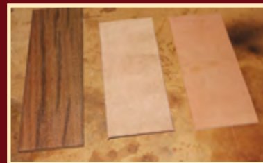
Timber blanks and leather pieces are pre-cut to final dimensions, laid out at the start of the strop-building process.
