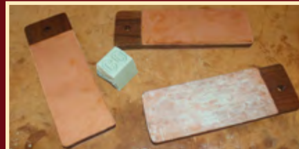
Compact paddle strops sized to slip easily into a hunting pack – ideal for family and friends on the move. The suede faces have been charged with polishing compound, ready for final honing.
