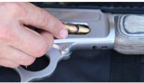
Loading the Marlin through the side loading gate, using the previous round to hold the gate open.
