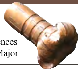
Barnes Triple-Shock 130-grain .270 Winchester projectile found embedded in a tree after fully penetrating the chest cavity of a harvested fallow deer.
