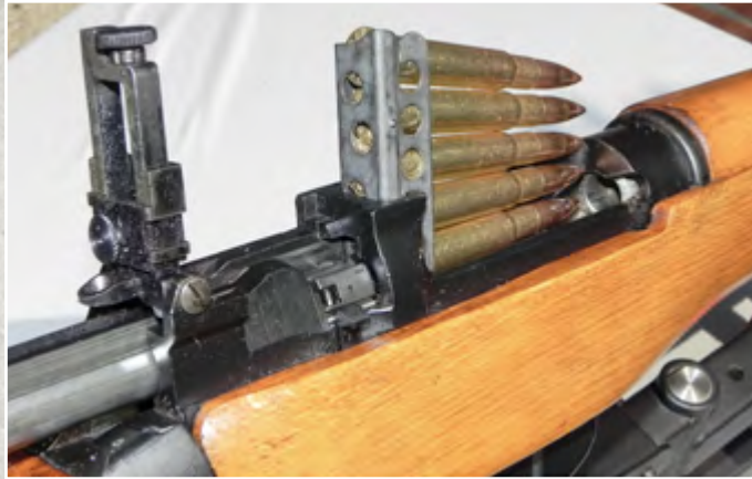
A Lee-Enfield No. 4 Mk 2 with a ladder aperture sight flipped up and a five-round charger in place to push down into the magazine. (British Army)
