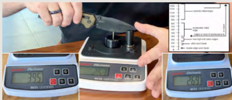
BESS professional sharpness test performed to test edge retention and ease of sharpening.
