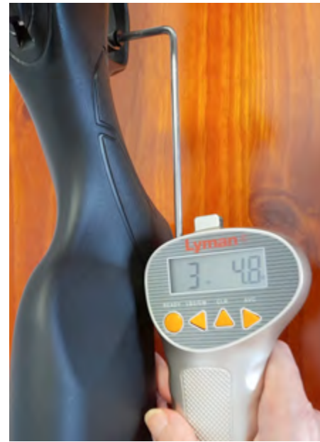
The author is very happy with the trigger pull weight on his Lithgow LA102.243, which ranges from 3lb 2.1oz to 3lb 4.9oz.
