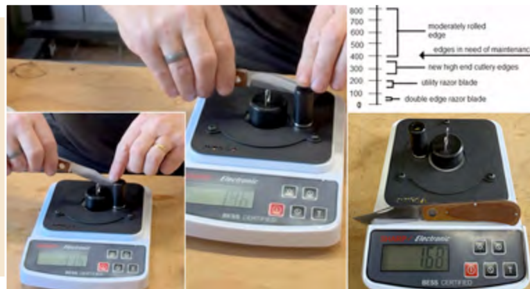
BESS professional sharpness test performed to gauge edge retention and ease of sharpening: 196g new, 315g after all testing, 168g after quick re-sharpen.
