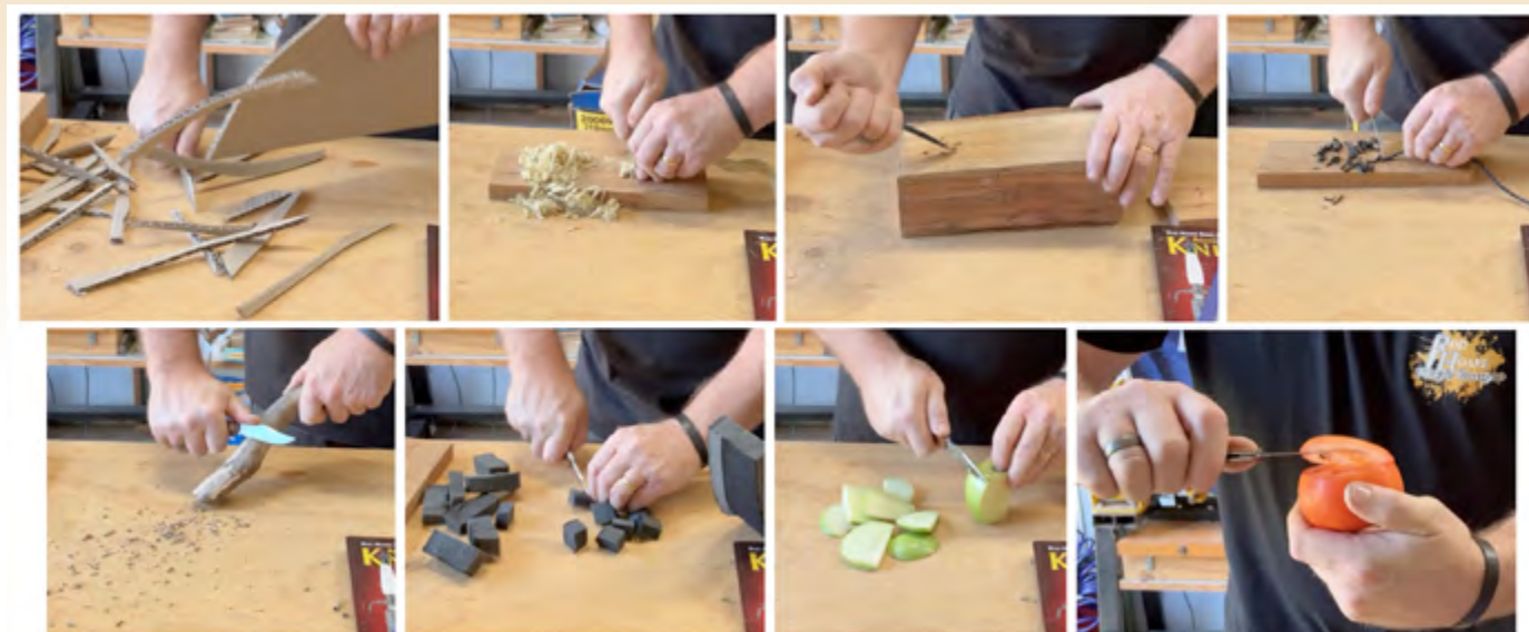
Performance testing to gauge edge retention, strength, comfort and durability, in order of testing L-R: heavy cardboard cut, sisal rope cut, tip strength bend test, nylon rope cut, shaving hardwood, foam cut, apple/tomato cut.
