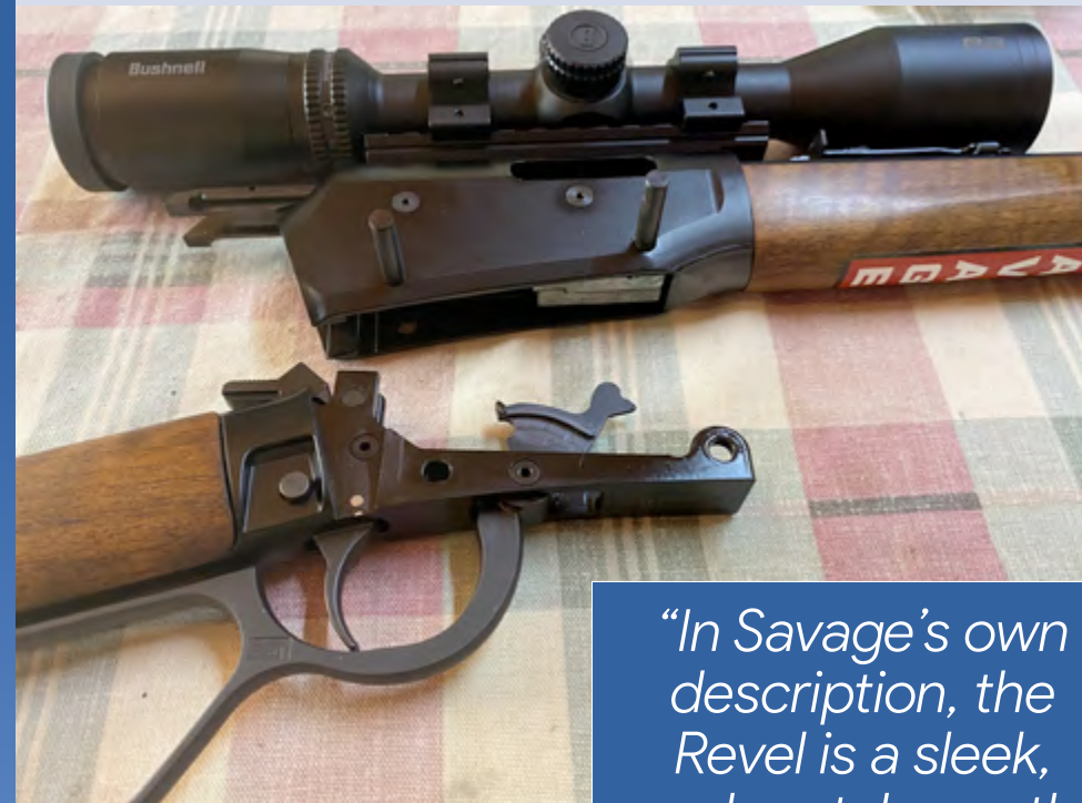
The Revel is easily taken down into its two major component parts by pushing the captured retaining pins through the action.
