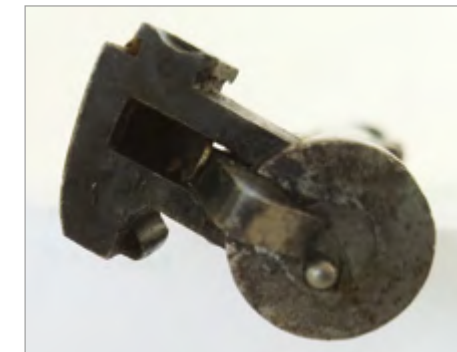
The bolt face has been modified by replacing centrefire firing pin with an offset rimfire firing pin.
