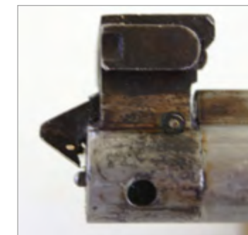
This image shows the original .303 extractor modified for .22 rimfire.
