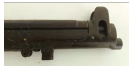
The original forewood has been shortened and modified to take an SMLE nose cap.
