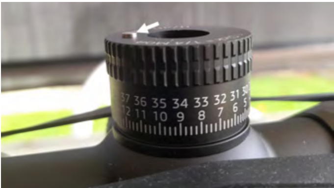
The stainless-steel post that pops up on the second rotation of the turret.
