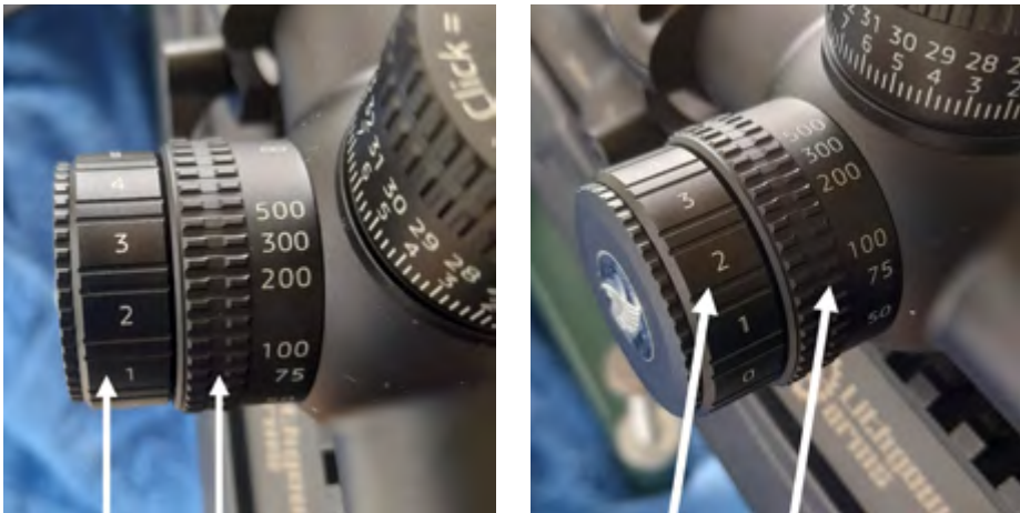
The third turret incorporates the parallax adjustment and red dot illumination controls.
