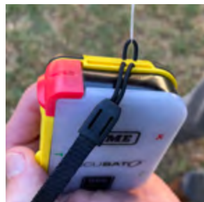
A trick to easily attach the lanyard to the PLB is to use a bit of dental floss to pull the strap through.
