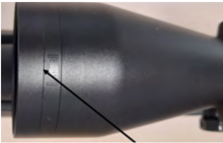
A loose objective lens cap blurred the target image at 100 metres.
